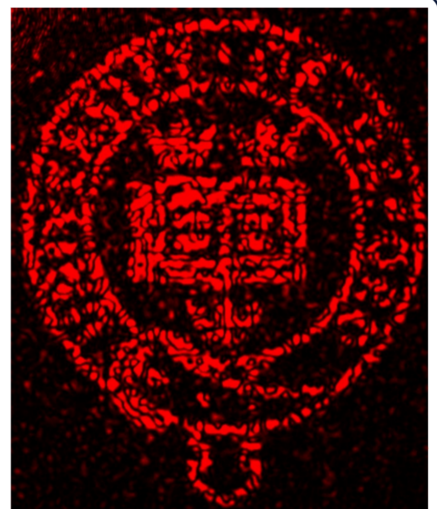
A projection of the Oxford crest using a hologram written into a liquid crystal device.
