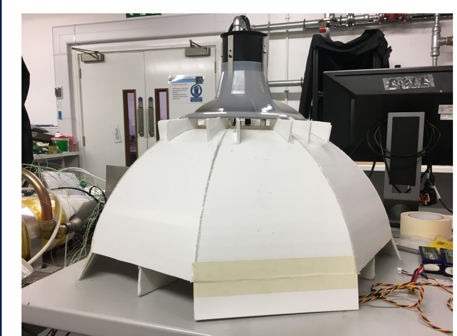
Figure 3: Photograph of the drone taken on 31 Jan 2020. Foam board vanes inserted to ensure uniform duct height.
