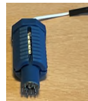
The dry electrode, in a screw-spring housing. Prongs are 2 mm.
