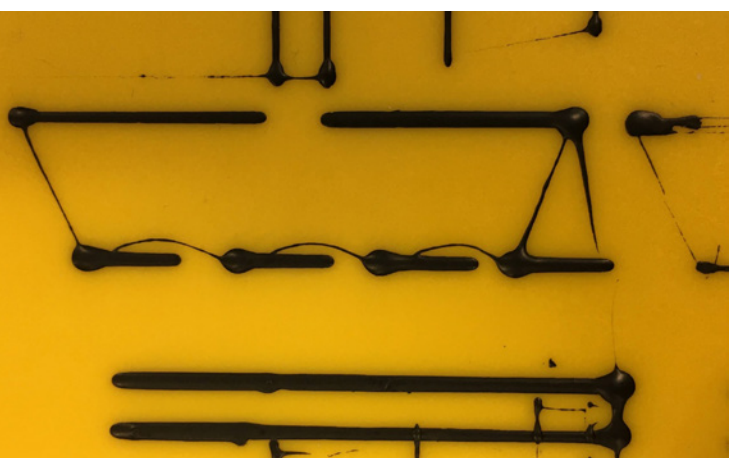
Photo of line prints where not enough paste was retracted.
